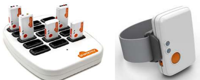
Figure 4: Shimmer Consensys base (left) , Shimmer3 wireless unit IMU (right)
