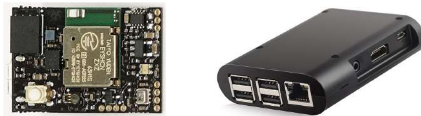
Figure 5: MetaMotionR board(left) and MetaHub device (right)
