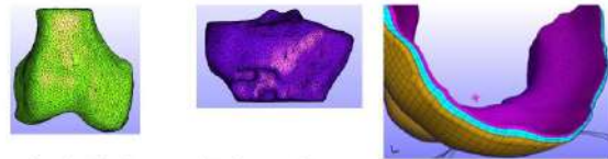
Femoral cartilage layers grouped into three zones that permits the assignment of different material properties to model different cellular synthesis
