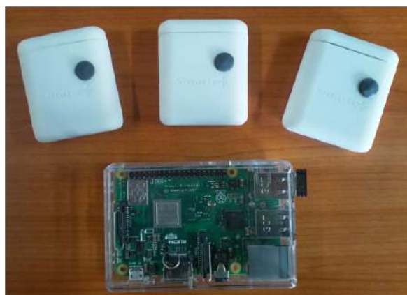
Figure 9: IMUs devices and the Raspberry Pi bridge
