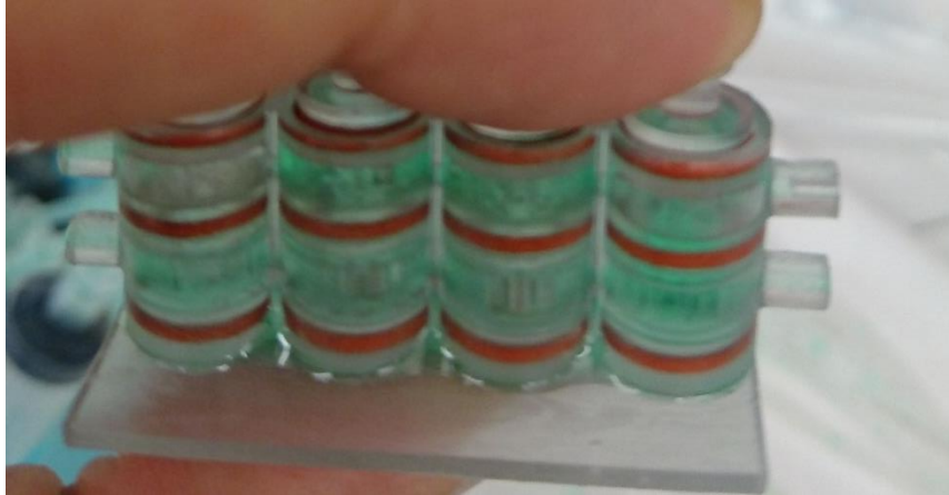
Figure 6: Leaking issue affecting a bioreactor
